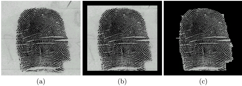
Fig. 2. Fingerprint image showing the effect of the masking operation; (a) original image; (b) 30 pixel wide strip along the borders; (c) mask over the image. Singularities located in the black area are not considered in the classification process.
